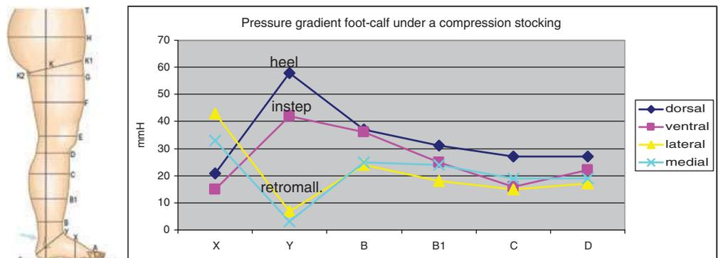
**Figure 3.** Pressure measurements under a compression stocking performed on the dorsal, ventral, medial and lateral aspect of the foot (X), the ankle (Y) and the lower leg (B–D) using a circular pressure probe of 45 mm diameter (Picopress®) (HP). On the foot (segment X) the highest pressure is measured over the lateral and medial edge of the foot and the lowest over the flat parts (dorsum and foot sole) according to the law of Laplace.
