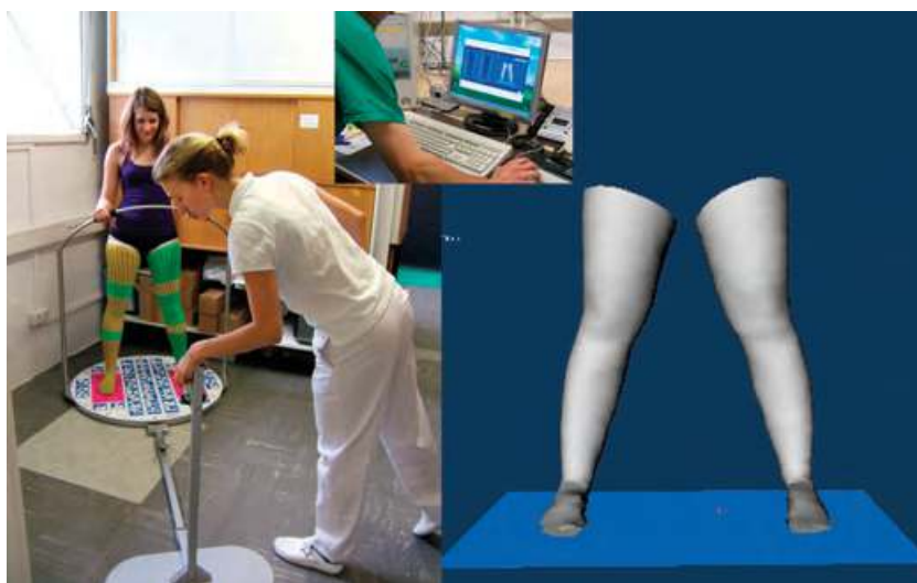
Figure 3: Volume of the legs measured by Image-3D-system (Fa. Bauerfeind). A digital camera takes photos of the leg at different points. A computer calculates an exact 3D model of the leg with the corresponding measurements.
